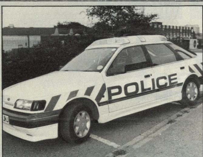
Woodway Engineering, which specialises in automotive lighting, has unveiled a new roof lighting system for police and other emergency services vehicles. Called System 2000, it has been designed to replace light bars strapped onto car roofs. It can be wired into the car's standard power system, without special fixings. Woodway can be reached on 0203 617242.
